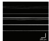
Left: Individual layers (horizontal lines represent interfaces) and pixels (squares in the middle of the images) of a smartphone.\*
