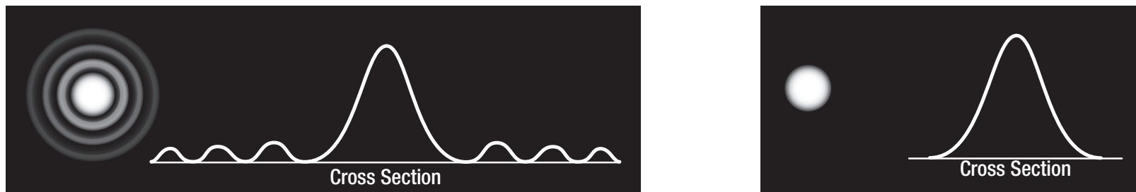
Figure 12: Apodization changes the intensity profile of the optical signal. In this case, apodization is used to filter the structure surrounding the central spot (left) and transmit only the center portion (right).
