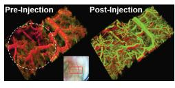
3D OCT image from a blood vessel network in a mouse ear before (left) and after (right) the injection of a contrast agent. The inset shows a photograph of the mouse ear: the scan area is highlighted by the red box.1
