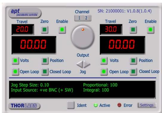
Fig. D.1 Piezo Controller GUI panel (dual channel version)
