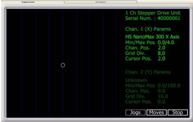
Fig. 4.6 Motor GUI Panel - Graphical View
