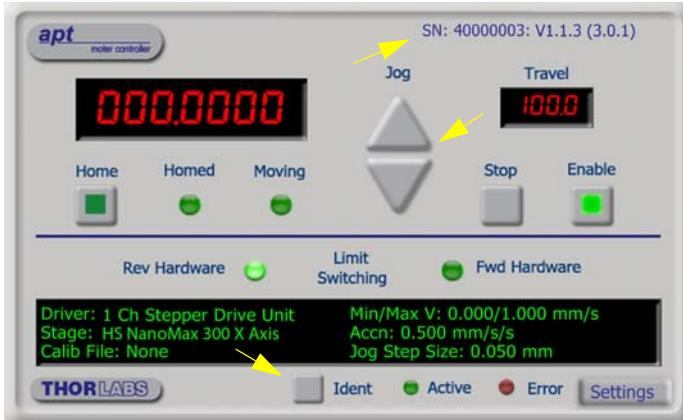
Fig. 3.4 Gui panel showing jog and ident buttons
