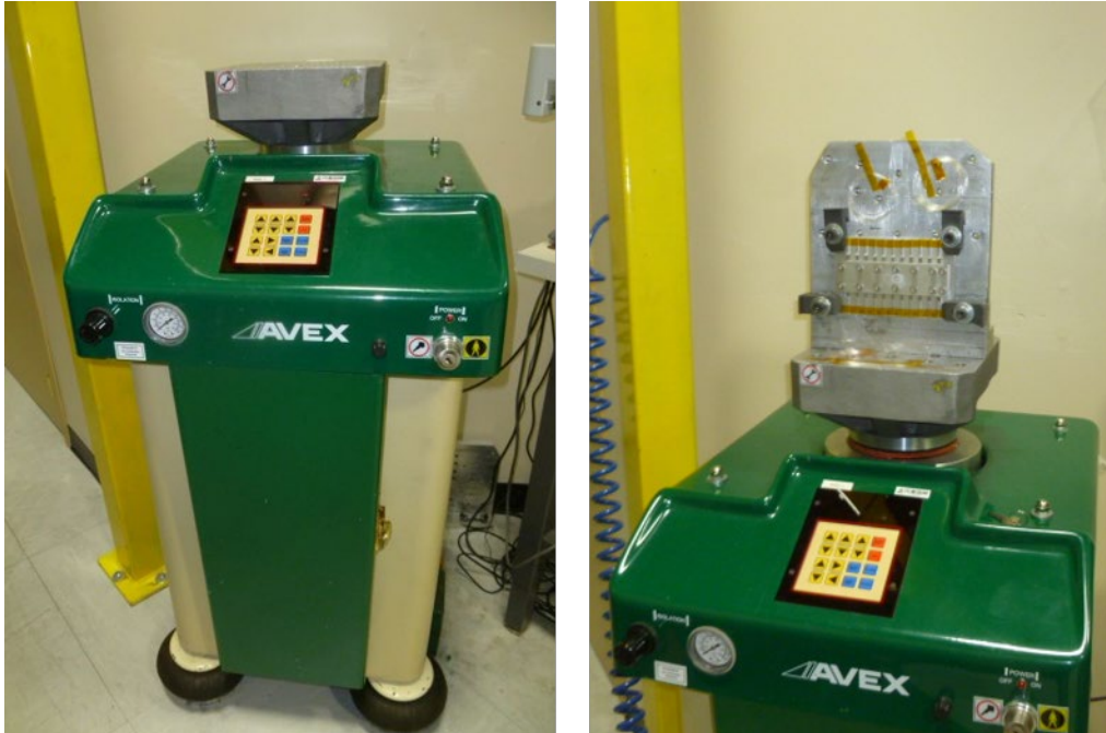
Figure 2 Mechanical Shock Test Setup
